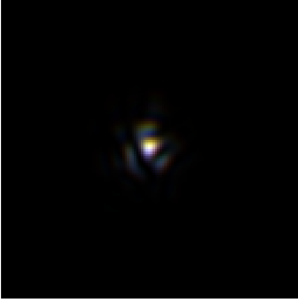
Figure 4: Simulated short exposure image through an AT pointing at the zenith with 4r_0 across the aperture diameter.
