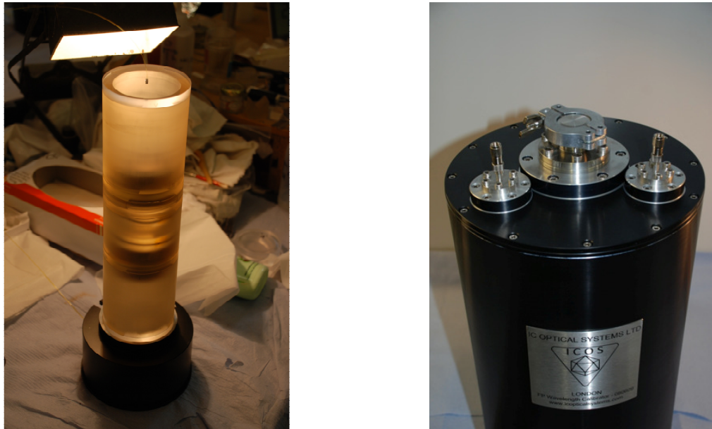
Figure 3: L/h: FP etalon and glass work . R/h Vacuum vessel containing the FP etalon and glass work
