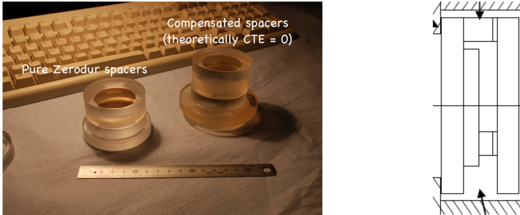
Figure 3: L/h The two Fabry-Pérot etalons produced. Pure Zerodur-spacers etalon of low CTE (spare) and etalon with compensated spacers for theoretical zero CTE (in service). Conceptual view of the thermally compensated etalon spacer. The vertical arrow at the top shows the compound spacer. The arrow at the bottom point to the additional fused silica plate. The thermal expansion of the spacer matches that of the silica plate.
