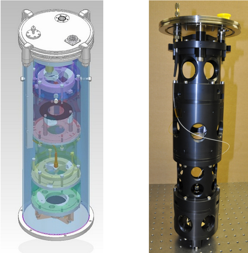
Figure 2: The latest opto-mechanical structure of the FP calibrator. L/h CAD view. R/h the assembly in the integration lab, with the vacuum enclosure cover already mounted. This design allows the fibers to be mounted on FC connectors and changed easily if need. Moreover, the connector base can be aligned with screws and shims to give the best focusing and the best coupling.
