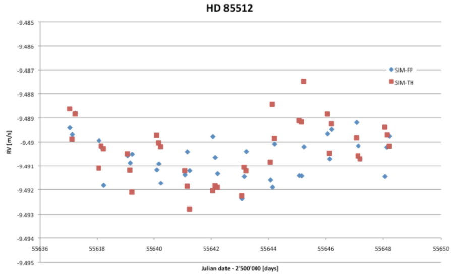
Figure 8: Observations of the star HD 85512 over a ten-days period with the simultaneous reference technique using the Th-Ar (red) and the FP system (blue). Radial-velocities are identical; although the dispersion seems to be even a little bit lower when using the FP system
