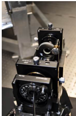
Figure 10. The focal plane module. From the left to the right on the L/h figure (resp. bottom to top on the center image): The artificial star+fiducials ferrule, the pupil alignment mask, the pick-off mirror for the photometer in the super stable source feedback loop and the apodizer. The R/h picture shows the focal plane ferrule with the central star and the four fiducials. The dot at the bottom right is the fiber collecting the light from the pick-off mirror. The screws are holding the anti-reflection mask need to control ghosts.
