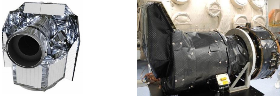
Fig 1. Artist view of the CHEOPS satellite L/h, CHEOPS instrument STM during AIV R/h.
