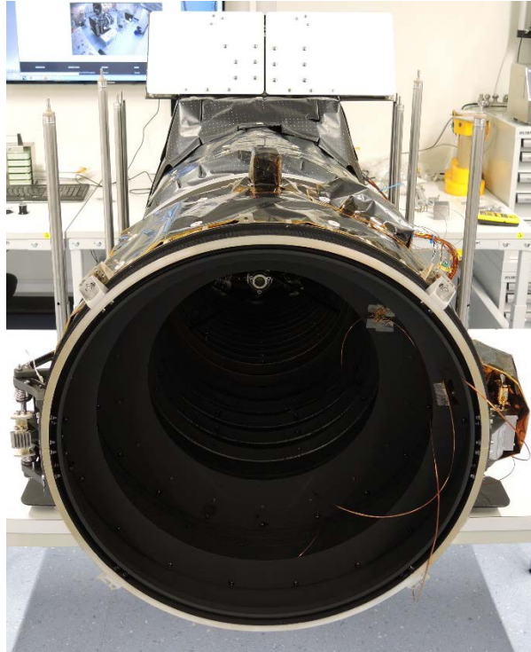
Fig. 4. Picture of the structural thermal model of the BCA and OTA seen from the front side.
