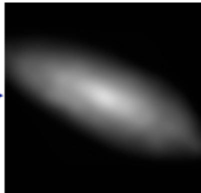
Atmosphere and telescope cause a convolution
