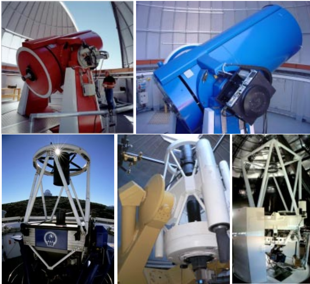
Figure 5.1: The five telescopes involved in the COSMOGRAIL project. From left to right, and top to bottom: (1) the Swiss 1.2m Euler telescope located at the European Southern Observatory of La Silla, Chile, (2) the Swiss-Belgian 1.2m Mercator telescope located on the Canarian island of La Palma, Spain, (3) the 2m robotic telescope of the Liverpool University (UK) also on La Palma, (4) the 1.5m telescope of the Maidanak Observatory in Uzbekistan, (5) the 2m Himalayan Chandra Telescope of the Indian Astronomical Observatory in Hanle.
