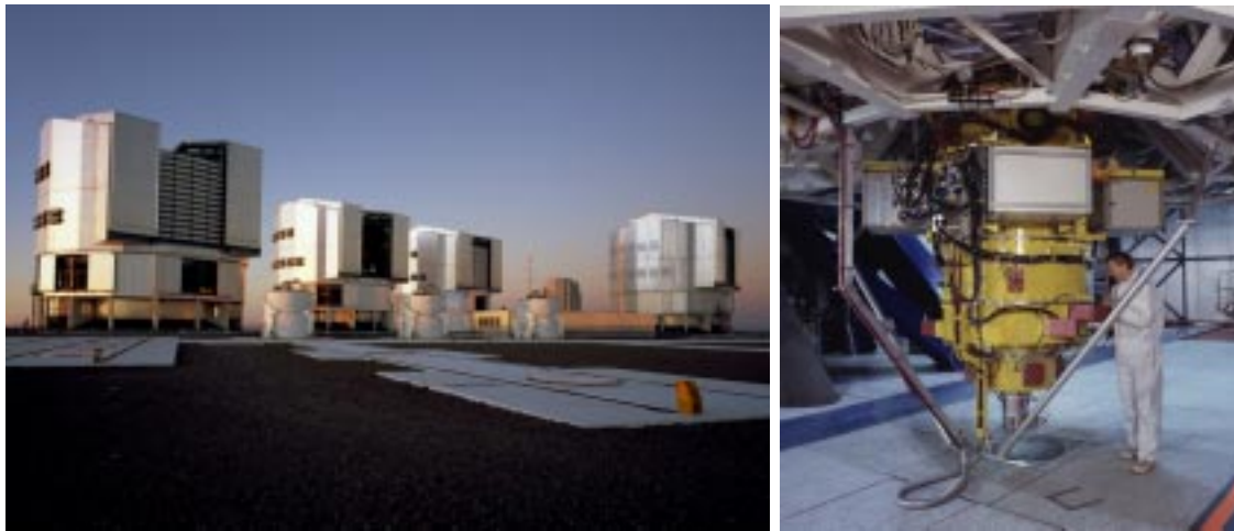
Figure 6.4: Right: The four 8m telescopes of the Very Large Telescope (VLT) of the European Southern Observatory (ESO) located at Mount Paranal, Chile. Left: The FOcal Reducer and low dispersion Spectrograph (FORs1) mounted on Kueyen, the second Unit Telescope (UT2) of the ESO-VLT. Image credit: ESO.
