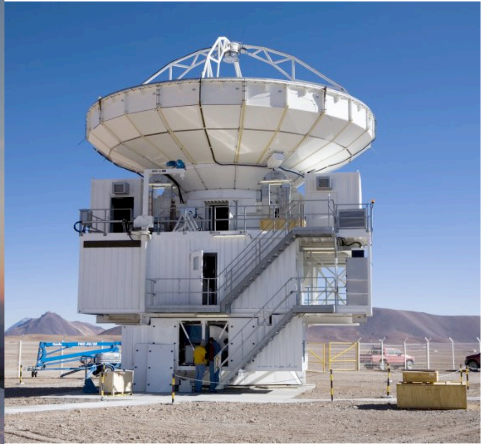
APEX 12m telescope (Chajnantor, Chile), altitude 5100m, surface accuracy 17 \mu\text{m}
