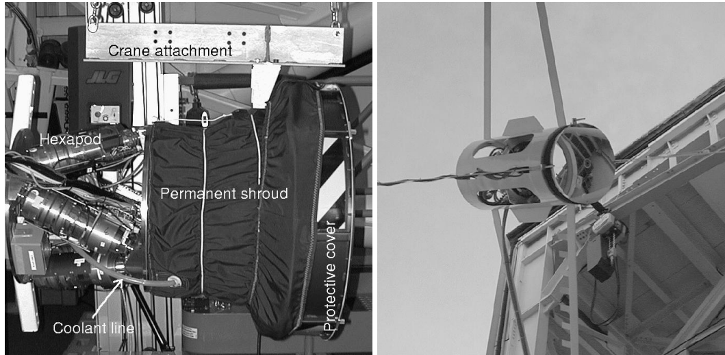
Fig. 1. The ASM ready to be lifted into the telescope's secondary hub (left) and mounted on the MMT (right).
