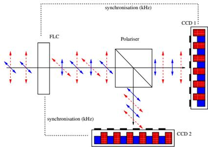
Figure 1. Measuring principle of ZIMPOL. The vertically polarized light passes the FLC where it is modulated into a time dependent polarization signal. The polarizing beam-splitter separates the two polarization directions into two time dependent intensity signals. The demodulation with the two CCDs is synchronized with the FLC.
