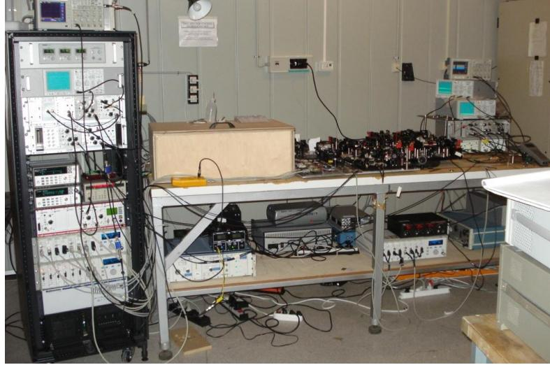
Fig. 5. LFC setup in January 2009 on HARPS. The Yb-doped fiber laser system is contained in the wooden box on the left hand side of the table, control and diagnosis electronics are in the rack and the breadboards with the Fabry-Perot cavities and amplifiers on the table. The LFC light is injected in the HARPS calibration box using an optical fiber .
