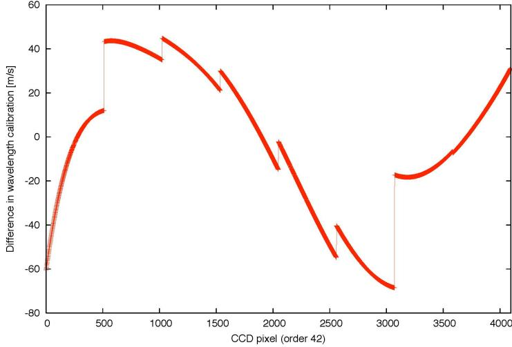
Fig. 7. Difference in wavelength calibration between standard Th-Ar and the LFC for echelle order 42.
