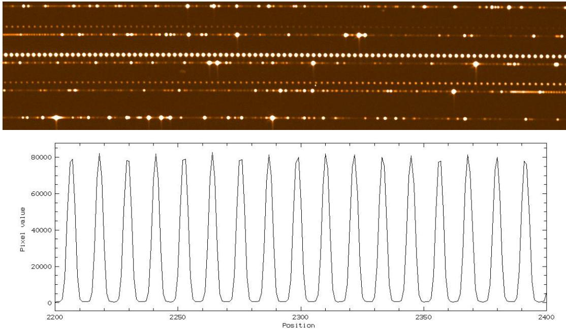
Fig. 6. Portion of the echelle spectra obtained during the test on HARPS. The spectrograph projects the signal from two fibers: one with the LFC signal, which is easy to identify in the image (row of equidistant dots) and whose cut profile is presented in the plot below, and the second with the Th-Ar spectra. The mode spacing for the LFC signal shown above was 18GHz. The graph on the bottom shows the LFC as sampled by HARPS
