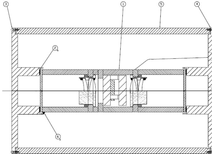
Fig 2: FCPS assembly. The outer structure is the aluminum vacuum cell. The internal closely dashed structure in the center is made of zerodur. It is optically contacted and hold all the optical components together. Light from an optical fiber enters on the L/h side, is collimated by the L/h triplet, goes through the etalon and is refocused by the R/h triplet on the fiber exiting on the R/h side. The assembly is meant to work vertically unlike shown on this figure.
