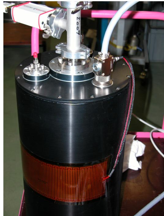
Fig 3: The FPCS in operation. The system is completely enclosed in the vacuum container. Light enters and exits the system via fiber optics feedthroughs. The heating pad seen on the bottom is part of the thermal control loop
