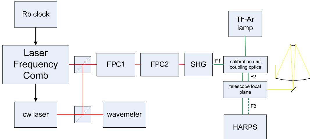
Fig. 4. The Laser Frequency Comb was filtered with two Fabry-Perot cavities (FPC1 and FPC2) to have a mode spacing of 18 GHz, and then frequency doubled (second harmonic generator, SHG) to a center wavelength of 514.9 nm. LFC light is injected in the calibration unit using fiber F1. From the calibration unit, two fibers (F2) brings, one the comb light and the second the Th-Ar. Using two F3 fibers, comb and Th-Ar signals are delivered to the HARPS spectrograph.
