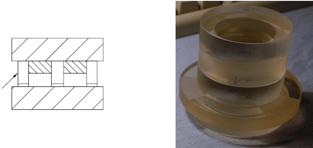
Fig 1: Plan of the compensated etalon. All dashed parts are fused silica plates. The vertical expansion of the center plate matches that of the 2-part etalon spacer ( $L/h$ ). On the picture on the right, one can see that the etalon is already mounted on a structural zerodur plate that is part of the mechanical structure of the system.
