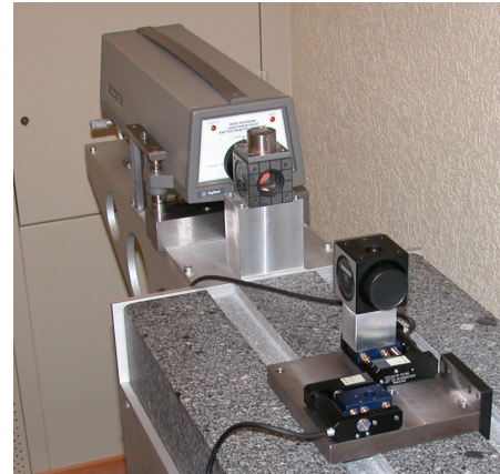
Fig 5: Characterization of each precision motorized stage used for phase diversity measurements was performed with an interferometer (R/h). After hysteresis correction the error curve shows a significant residual at a frequency of 0.5/\text{mm} , a sub-harmonic of the pitch of the lead screw of 2/\text{mm} that would prevent reaching the required accuracy. The stages were finally characterized between 2 fixed positions, with sub-micrometer repeatability.
