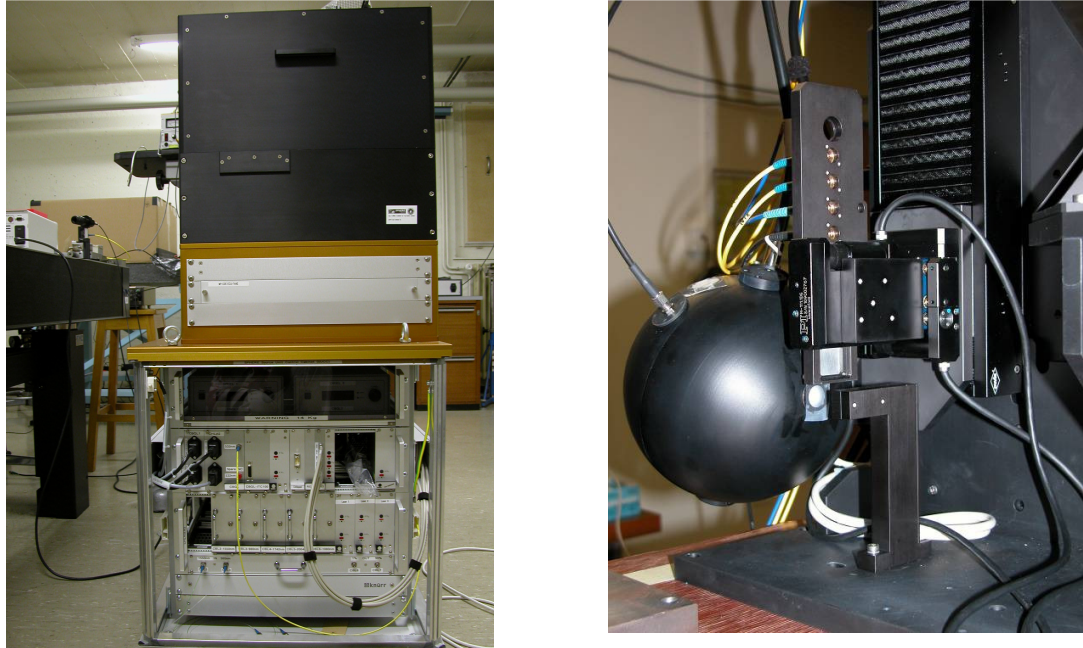
Fig 9: Photographs of the source unit (L/h) and the main feed unit (R/h) of the calibration module. The point sources on the feed unit are mounted on an horizontal stage (Z-axis) to allow re-focusing when the polarization components are inserted in the beam, which changes the location of the SPHERE input object point. X and Y motions allow for precise centering on the coronagraphs. The SPHERE field stop can be seen above the fiber point sources. Once fully integrated, this assembly is almost hidden behind the rotating half-wave plates of the polarization mode.
