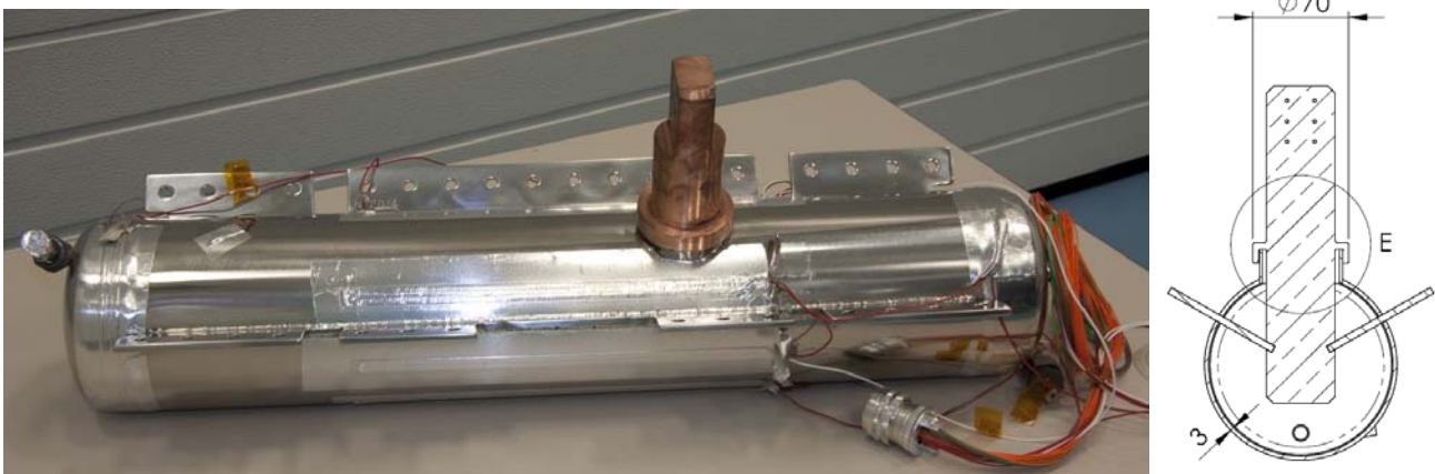
Figure 7. The small LN2 tank (left image), known as the submarine, takes the form of a long cylinder situated under the optical bench. Cooling braids are fixed onto the wings. A copper rod provides cooling power to the detector. The design of the soldered junction between the rod and the stainless steel tank is made to ensure its viability through numerous cooling cycles (right image).
