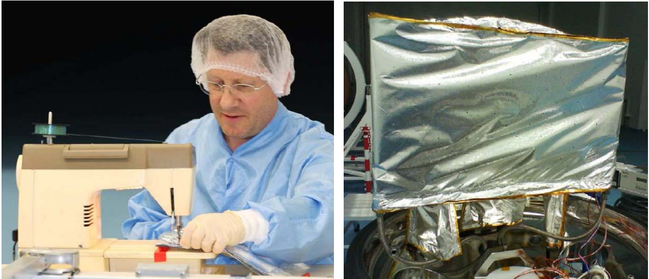
Figure 6. Manufacturing of the multi-layer insulation (MLI) coat (left image) and the coat covering the main LN2 tank and hexapod structure installed (right image).
