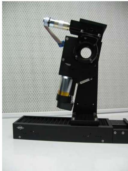
Figure 5. Implementation of the Polarization Compensator
