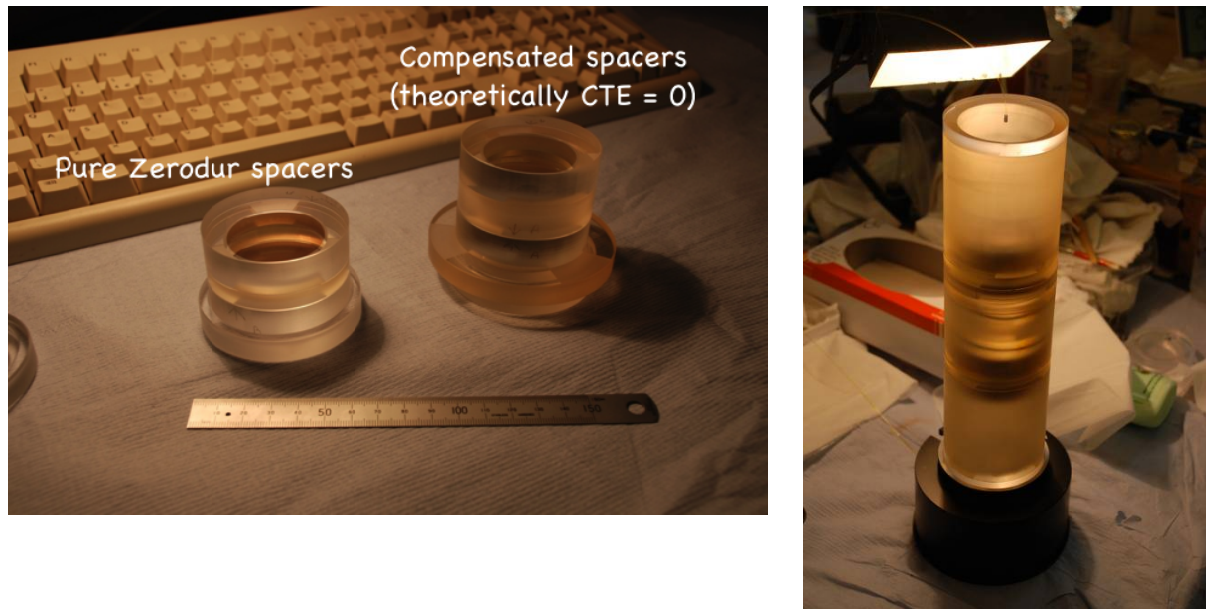
Figure 2: L/h The two Fabry-Pérot etalons produced. Pure Zerodur-spacers etalon of low CTE (spare) and etalon with compensated spacers for theoretical zero CTE (in service). R/h: assembled Fabry-Pérot ‘glasswork’. The system is completely optically contacted within a Zerodur support structure. The lenses are mounted inside the structure as well
