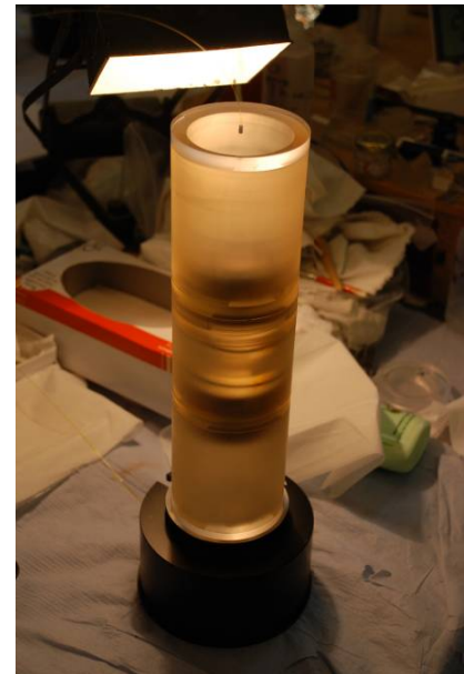
Figure 2: L/h The two Fabry-Pérot etalons produced. Pure Zerodur-spacers etalon of low CTE (spare) and etalon with compensated spacers for theoretical zero CTE (in service). R/h: assembled Fabry-Pérot 'glasswork'. The system is completely optically contacted within a Zerodur support structure. The lenses are mounted inside the structure as well
