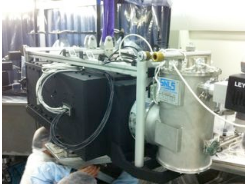
Figure 10: IFS mounted on the SPHERE huge bench. Close up is the IFS Dewar.
