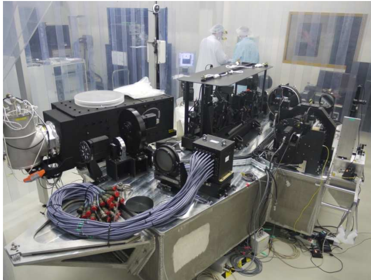
Figure 10: SPHERE optical bench, on the ground for SAXO components integration and alignment. Bottom front: HODM is visible, on the left, black box is IFS.
