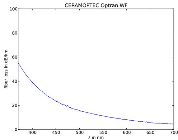
Figure 3: View of the fiber transmission across the wavelength range of HARPS-N. For a 25 m fiber the maximum loss is ~ 25 % at the extreme blue part of the spectrum.
