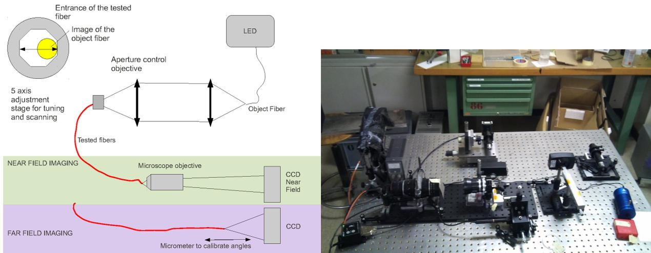
Figure 2: Scheme and actual photo of the fiber test bench.
