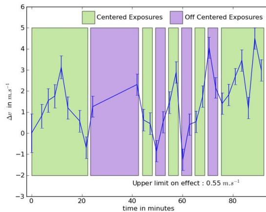
Figure 11: On sky test with HARPS-N: the star is observed, some exposure are made with the star centred (the purple zones) and other are off-centred (the star is on the border of the fiber). There is no obvious effect to be noted. An upper limit  $0.55 \text{ m s}^{-1}$  for the effect of decentering can be set. However this measure has not been done in an optimal way and the p-modes of the star are dominating all the effects.
