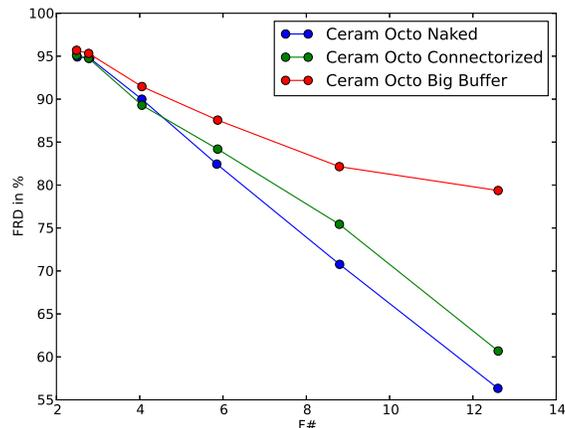
Figure 6: Compared FRD for 3 fibers: The octagonal fiber for HARPS-N, naked and connectorized and another octagonal fiber from the same company with a much larger cladding and buffer. The later has the best FRD we have ever measured. The fact that the naked fiber seems to have a worse FRD than the connectorized one is to be attributed to systematic errors in the measurements. One has to see they have a similar behaviour.
