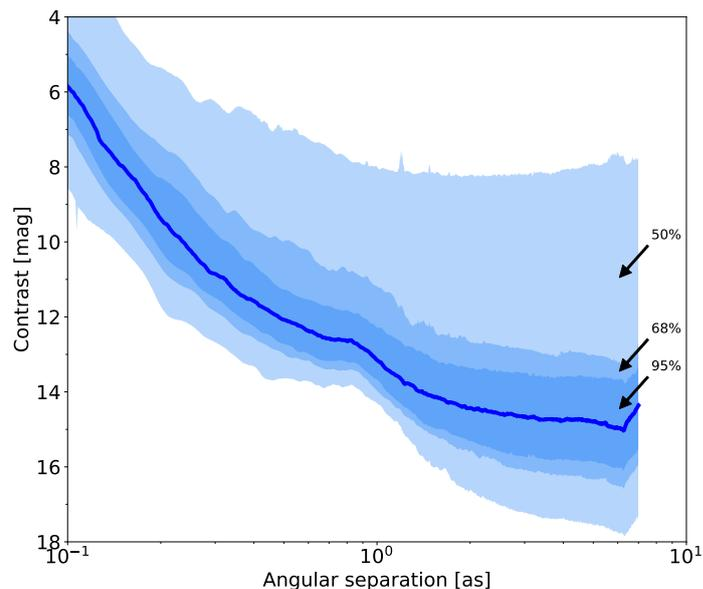
Fig. 22: Median  $5\sigma$  contrast achieved by IRDIS in DBI H23 mode (H2 ADI only) in 1h30 observing time on average with T-LOCI post-processing. The plain blue line represents the median, and the different shades of blue background represent the 95%, 68% and 50% completeness intervals.
