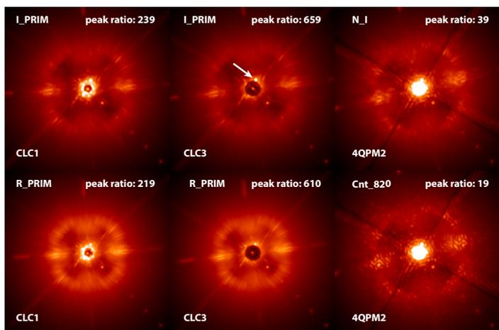
Fig. 13: Visible coronagraphic images (FoV =  $1.6''$ ) of HR 591 corresponding to the configurations of Fig. 12, together with fake planets at  $10^{-3}$  and  $2 \times 10^{-4}$  levels. The stellar companion  $\alpha$  Hyi B is indicated by an arrow.
