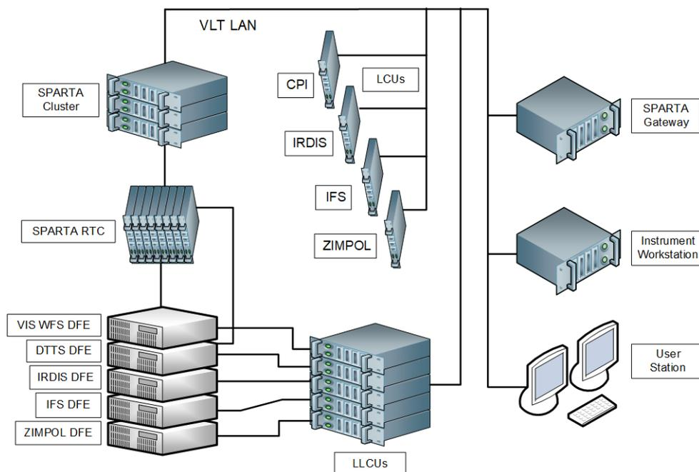
Fig. 26: Conceptual view of the SPHERE control network.
