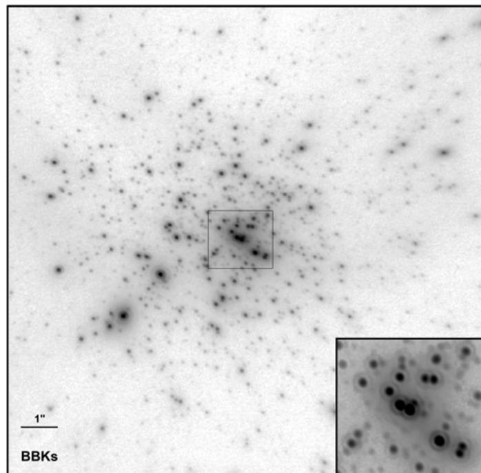
Fig. 25: Broadband *Ks* image demonstrating the PSF quality achieved by SPHERE using IRDIS CI mode without coronagraph in a field-stabilized observation. The bottom right inset displays a zoom image of the square box located at the center of the R136 open cluster (Khorrami et al. 2017).
