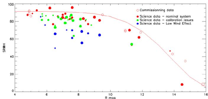
Fig. 7: Strehl ratio in  $H$ -band, measured on-sky during commissioning and science verification. The nominal performance are plotted in red circles. Different problematic regimes are also plotted in green and blue circles. The nominal trend is overplotted with a solid red line.
