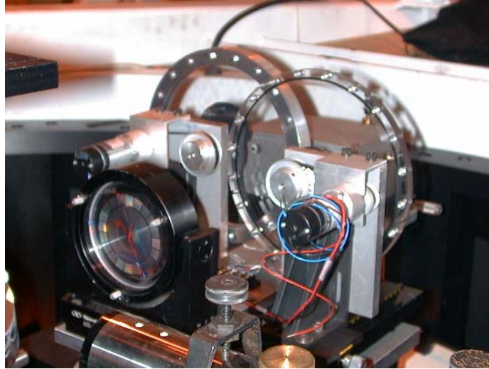
Figure 4. Arrangement of two spinning phase plates in the optical path of the shimmulator. They are machined acrylic plates filled with index-matching oil. At lower left is the computer generated hologram that removes spherical aberration from the shimmulator optics.
