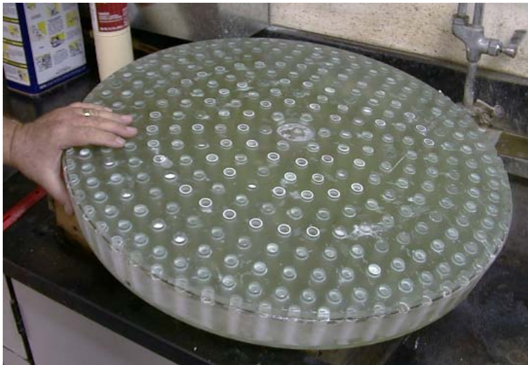
Figure 6. Glass reference plate for the adaptive secondary. The actuators project through the 336 holes piercing the plate. The thin mirror itself will be supported by the actuators above the top surface of this plate with a gap of 40\ \mu\text{m} .
