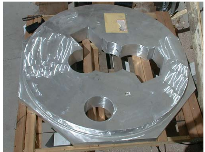
Figure 2. Shimmutator mechanical structure (left), showing the large fold flats and the unmounted top box on its handling cart. The top box (top right) is normally raised from its handling cart and mounted to the dummy rotator ring. (Lower right) the cast aluminum optics bed which forms the floor of the top box. The cutouts are designed to accommodate existing instruments.
