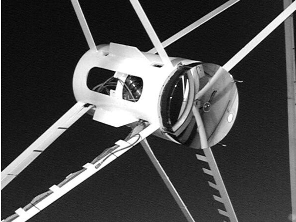
Figure 1. The adaptive secondary on the telescope. The photo was taken Jan 20, 2003 just before sunset at the MMT.
