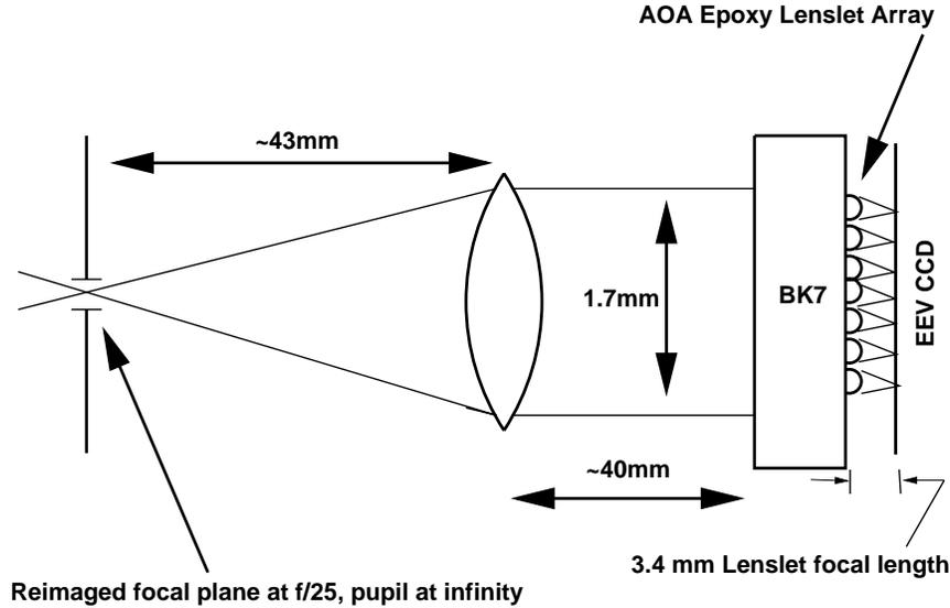
**Figure 2.** A sketch of the MMT WFS geometry (not-to-scale), showing the 2.5 arcsecond field stop in the  $f/25$  focal plane, the lens to form a pupil, and the lenslet array glued in close proximity to the CCD chip. plane
