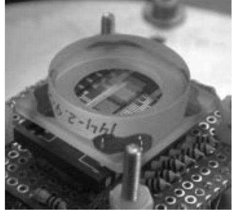
**Figure 3.** An assembled WFS after the lenslet has been bonded to the CCD package. Figure (a) displays a cross sectional diagram of the CCD, spacer, and lenslet. Figure (b) shows the WFS after assembly. The spacer for the WFS shown is made of BK7.
