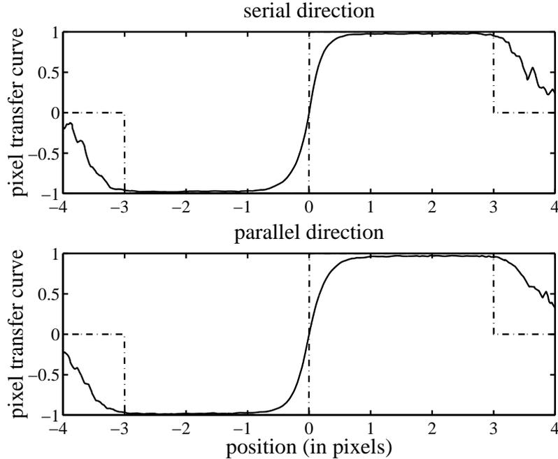
**Figure 6.** Pixel transfer curves between CCD pixels after binning by a factor of 3. The dashed line is for a perfect CCD with no pixel crosstalk and the solid line was calculated from the measured pixel responses. The top (bottom) graph shows the transfer curves for the serial (parallel) readout direction of the CCD. The units for the x-axes are pixel widths. The pixels are  $24 \mu\text{m}$  across.
